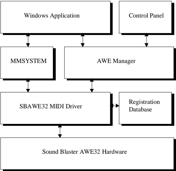
There are 16bit and 32bit (Windows NT) versions of SBAWE32.DRV to accommodate different applications in different platform. AWE Manager also supports both versions: AWEMAN.DLL for Win16 and AWEMAN32.DLL for Win32. The previous diagram shows the architecture which is common to both platform.
